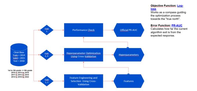
The diagram illustrates the training and testing process used for the machine learning model. Initially, the data is carefully sanitized, forming a 'Clean Base' with training sets for the year 2014, validation for 2015 and test for 2018. This www.imdsbrasil.org 11 of 18
